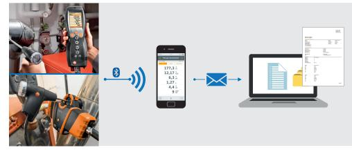
The measurement results of the testo 330-1/2 LX and the testo 330i LX are displayed in the App. From there you can send the measurement report by e-mail and archive it digitally on a PC.
